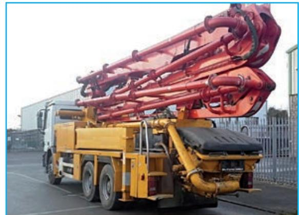
Fig 3: Truck Mounted Concrete Pump with Boom and Pipeline
